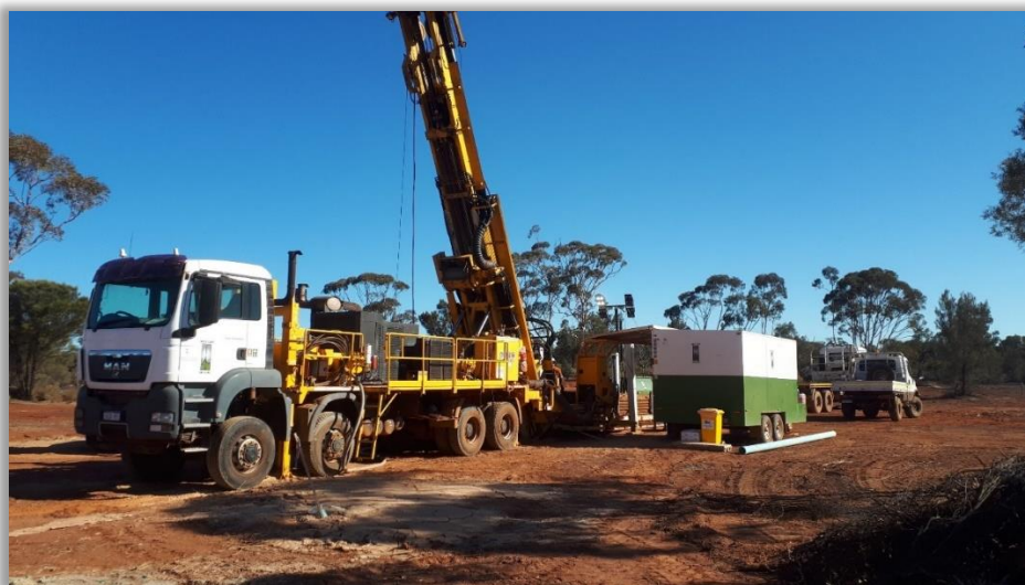
Figure 2: Diamond drill rig set up on first hole of seven-hole program at East Sampson Dam
