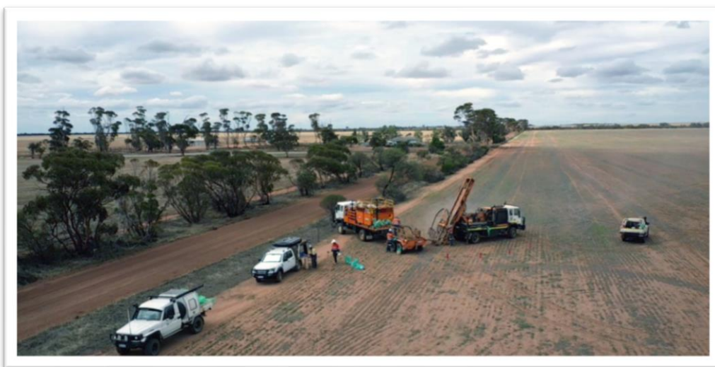
Figure 1: Air core drilling at Crossroads prospect with 'Low Impact Rig', Burracoppin Gold Project
